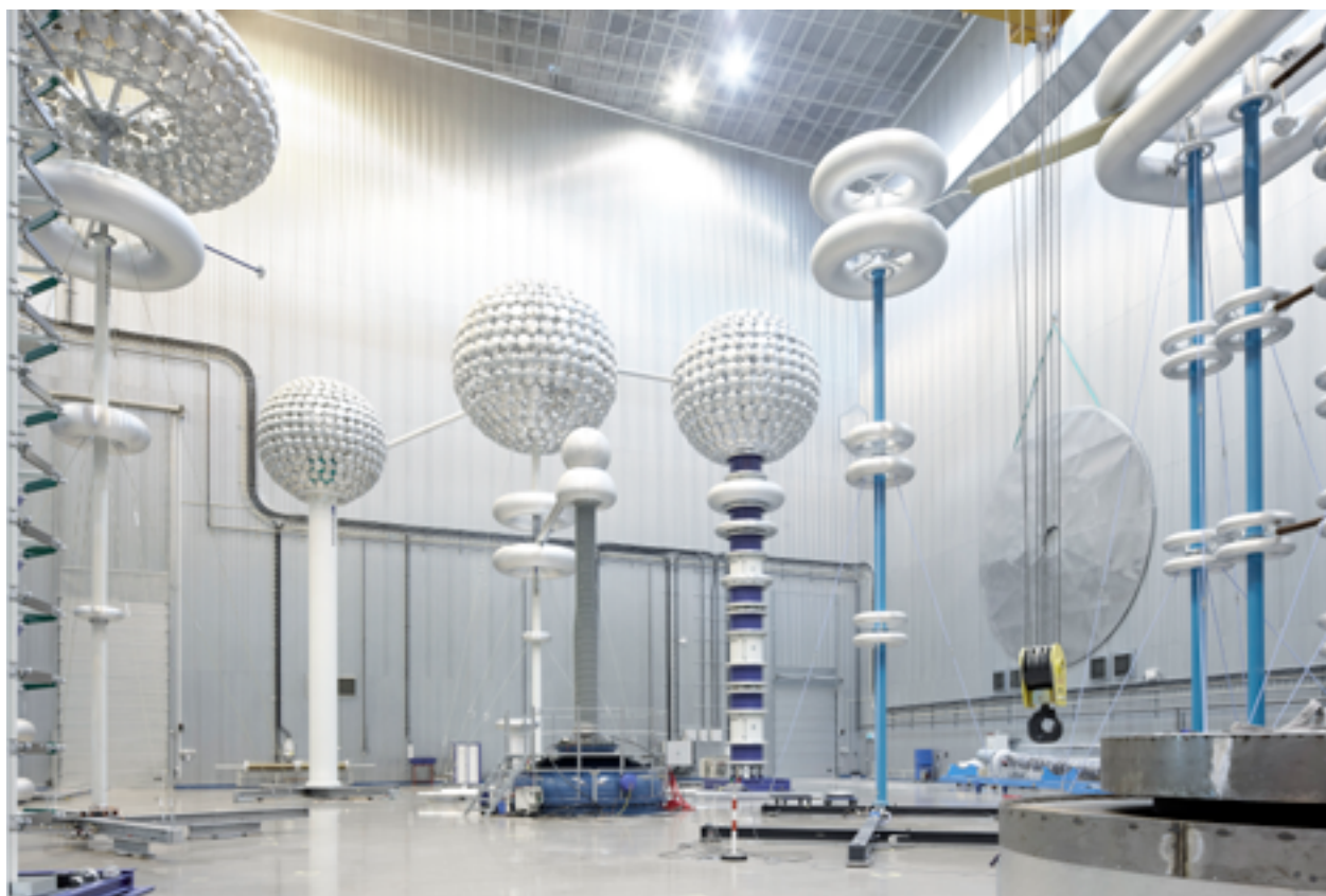
FIGURE 3. Hitachi Energy's ultra high-voltage test hall in Ludvika, Sweden, where the highest voltage products are tested for both AC and HVDC projects.
