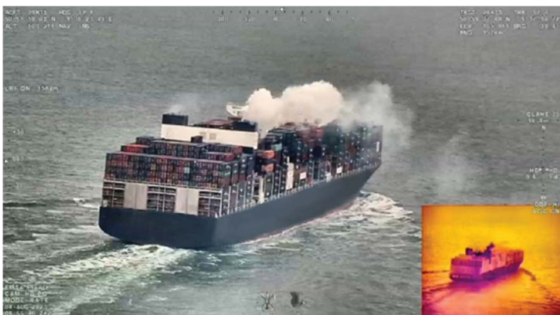
Figure 11 – Image from a drone approaching a vessel to measure the sulphur content of dense fumes
